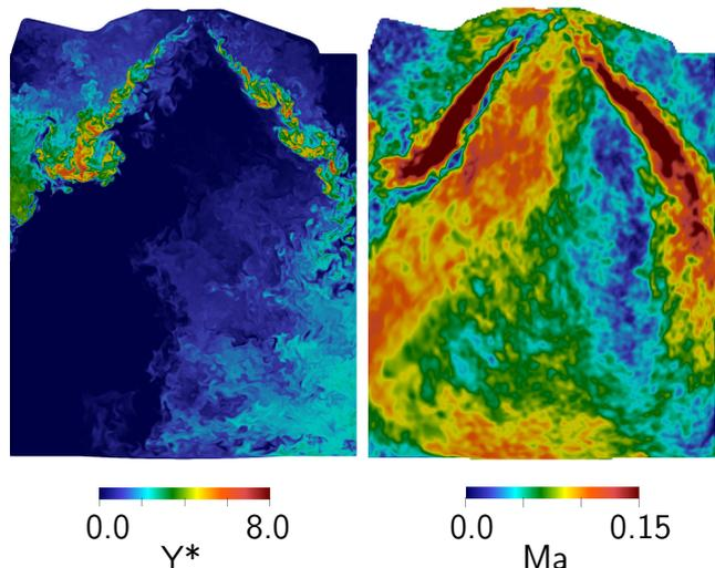
*Non-dimensional fuel vapor and mean Ma-number at the end of injection in the engine tumble-plane*
