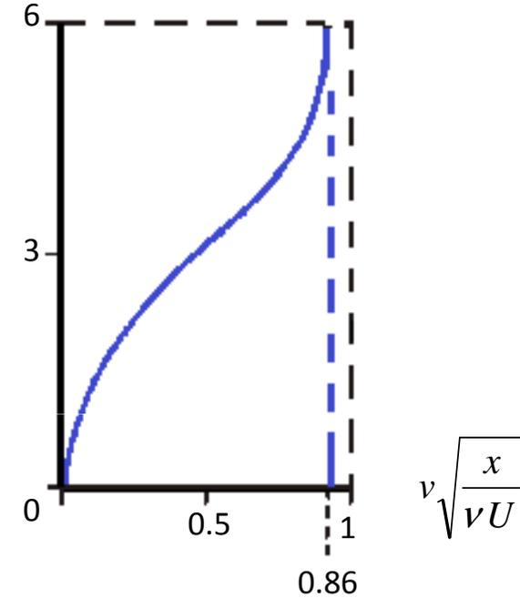
$$\begin{aligned} v = -\frac{\partial \psi}{\partial x} &= -U \frac{d\delta}{dx} [f - f'\bar{\eta}] & \frac{d\delta}{dx} &= \frac{1}{2} \sqrt{\frac{\nu}{xU}} \\ &= \frac{1}{2} \sqrt{\frac{\nu U}{x}} [\bar{\eta} f' - f] \end{aligned}$$
