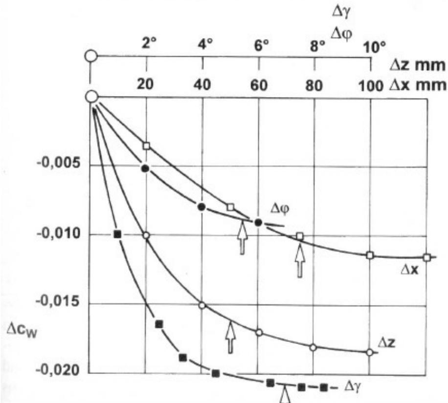
$$\Delta\varphi: \Delta c_D = -0.00472 \times \Delta\varphi^{0.36}$$
