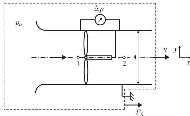
$$\begin{aligned} p_a &= p_1 + \frac{\rho}{2} v_1^2 \\ \Delta p &= p_2 - p_1 = p_a - p_1 \\ \implies \dot{V} &= v A = \sqrt{\frac{2 \Delta p}{\rho}} A \end{aligned}$$
