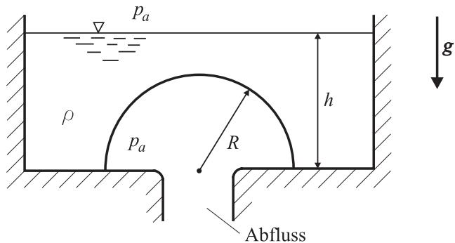
Determine the necessary force  $F$  to open the drain.
