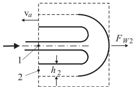
Momentum in x-direction:  $-\rho v^2 h B - 2\rho v_2^2 h_2 B = -F_{w2}$
