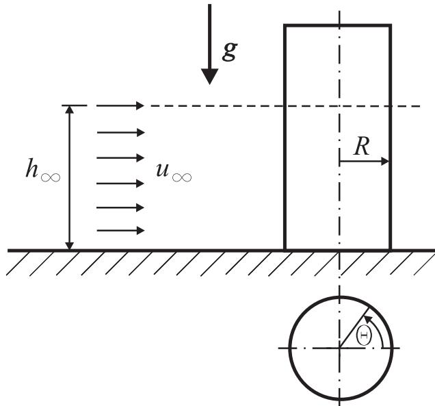
$$u_\infty = 1 \text{ m/s} \quad h_\infty = 6 \text{ m} \quad R = 2 \text{ m} \quad \rho = 10^3 \text{ kg/m}^3 \quad g = 10 \text{ m/s}^2$$
