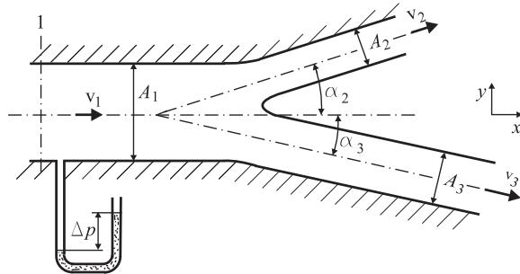
$$A_1 = 0,2 \text{ m}^2 \quad A_2 = 0,03 \text{ m}^2 \quad A_3 = 0,07 \text{ m}^2 \quad \alpha_2 = 30^\circ \quad \alpha_3 = 20^\circ \\ \Delta p = 10^4 \text{ N/m}^2 \quad \rho = 10^3 \text{ kg/m}^3$$
