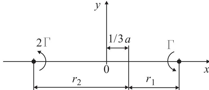
$$v_\theta = \frac{\Gamma}{2\pi r} : v_{\theta_1} = v_{\theta_2} \rightarrow \frac{\Gamma}{2\pi r_1} = \frac{2\Gamma}{2\pi r_2} \rightarrow r_2 = 2r_1$$
