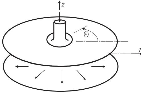
The flow is radial from inside to outside. The determining differential equations in cylindrical coordinates are
