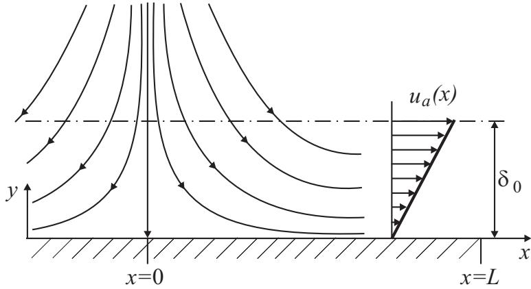
**15.9** The velocity profile of a laminar boundary layer in a flow along a flat plate (length  $l$ ) is approximated with
