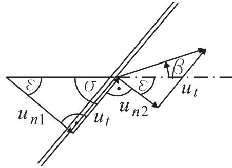
$$\begin{aligned} \tan(\beta + \varepsilon) &= \frac{u_t}{u_{n2}} \\ \tan(\varepsilon) &= \frac{u_t}{u_{n1}} \\ \implies \beta &= \arctan \frac{u_t}{u_{n2}} - \arctan \frac{u_t}{u_{n1}} = 12^\circ \\ \text{or } \beta \text{ from diagram } &\beta = f(M_1, \sigma) \end{aligned}$$
