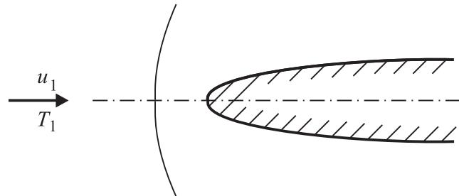
$$u_1 = 680 \text{ m/s} \quad T_1 = 287 \text{ K} \quad R = 287 \text{ Nm/(kgK)} \quad \gamma = 1.4$$
