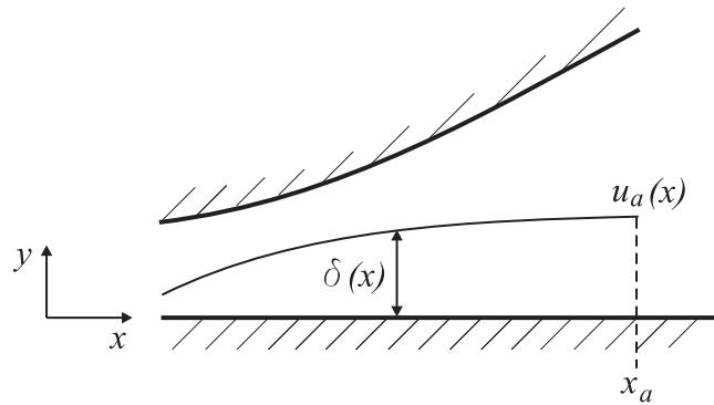
Determine the velocity profile  $\frac{u(x_a, y/\delta(x_a))}{u_a(x_a)}$  at the separation point.
