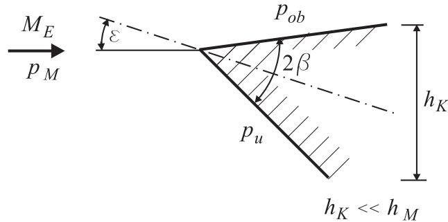
What is the maximum angle of attack  $\epsilon$  without the development of a detached shock? What is the pressure difference  $p_u - p_{ob}$  and the Mach numbers  $M_{ob}$  and  $M_u$  for this case?
