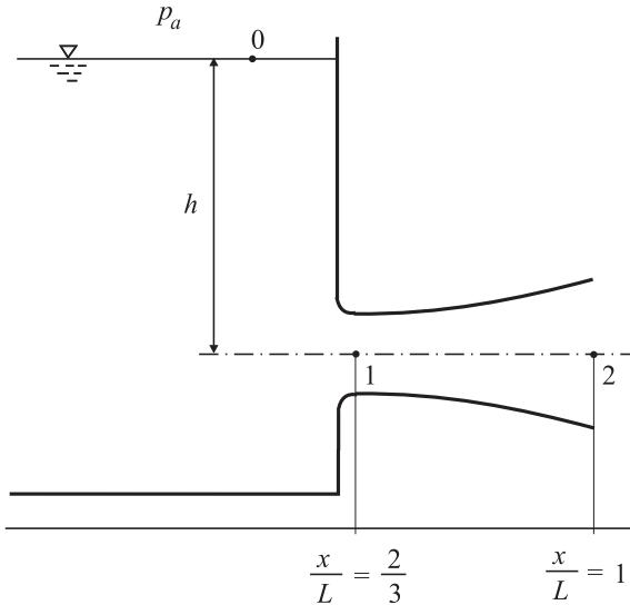
$$(1) \quad p_a + \rho g h = p_2 + \frac{\rho}{2} v_2^2 + \rho \int_{2/3 L}^L \frac{\partial v}{\partial t} dx$$
