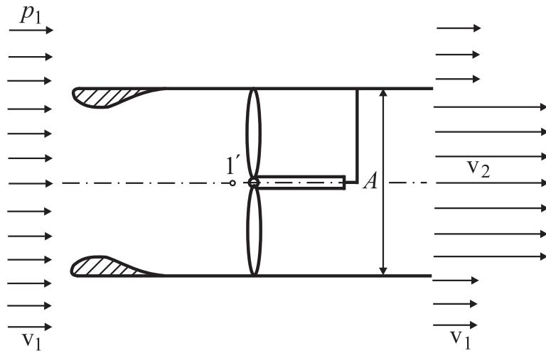
$$A = 1 \text{ m}^2 \quad v_1 = 10 \text{ m/s} \quad p_1 = 1,345 \cdot 10^5 \text{ N/m}^2 \quad p_{1'} = 10^5 \text{ N/m}^2 \quad \rho = 10^3 \text{ kg/m}^3$$
