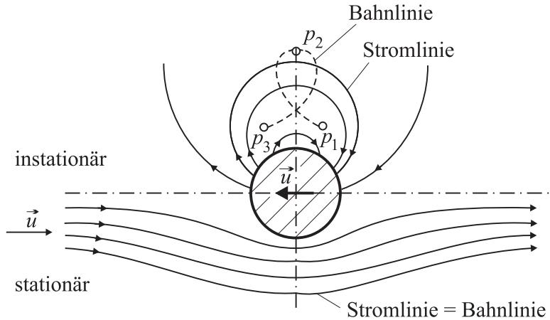
Unsteady flow for the resting observer, steady flow for the moving observer.
