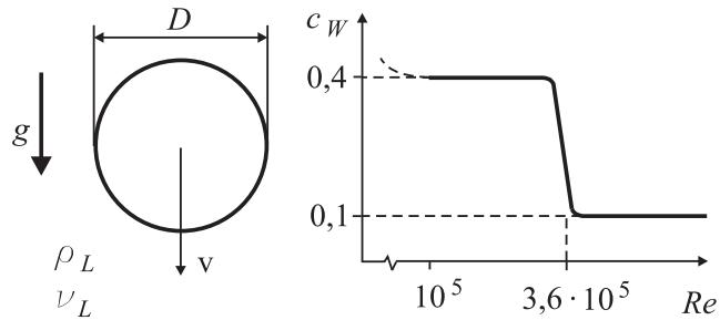
$$D = 0,35 \text{ m} \quad G = 4,06 \text{ N} \quad v_1 = 13 \text{ m/s} \quad v_2 = 18 \text{ m/s}$$
