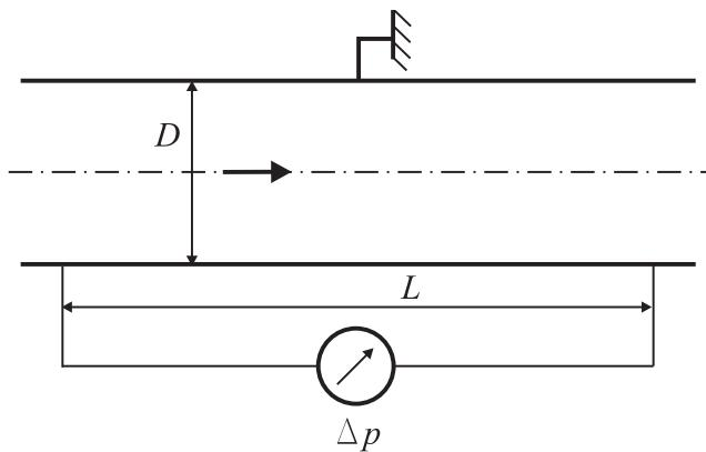
$$\begin{aligned}\dot{V} &= 0,393 \text{ m}^3/\text{s} & L &= 100 \text{ m} & D &= 0,5 \text{ m} & \Delta p &= 12820 \text{ N/m}^2 & \rho &= 900 \text{ kg/m}^3 \\ \eta &= 5 \cdot 10^{-3} \text{ Ns/m}^2\end{aligned}$$
