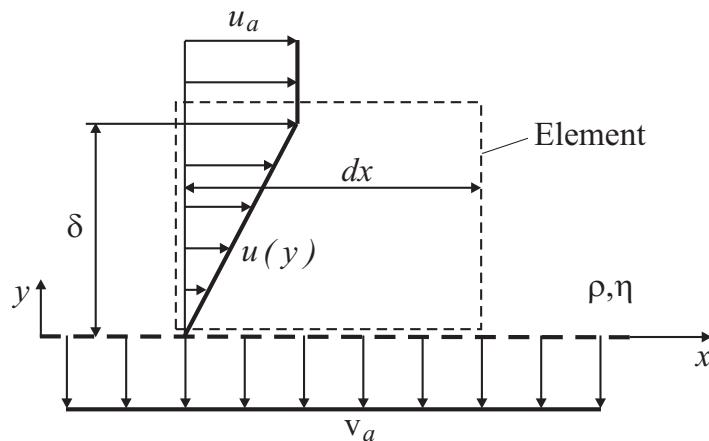
Determine the suction velocity  $v_a$  by using a balance for the sketched element under the condition that the boundary layer thickness  $\delta$  is independent of the length  $x$ . Assume that the tangential component of the velocity increases linearly.
