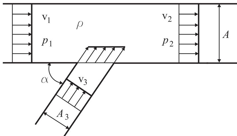
**7.3** Water is flowing through a bifurcation into open air stationarily. The pressure in the incoming tube is  $\Delta p$  higher than in the surrounding.
