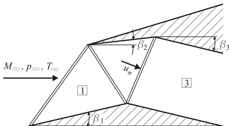
$$\begin{aligned} M_\infty &= 3 & T_\infty &= 270 \text{ K} & p_\infty &= 1 \text{ bar} & \gamma &= 1.4 & R &= 287 \text{ J/(kg K)} \\ \beta_1 &= 15^\circ & \beta_2 &= 10^\circ & u_n &= 649 \text{ m/s} \end{aligned}$$
