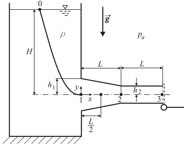
**6.7** The exit of a large container is build as diffusor. The flap at the end of the diffusor is opened at  $t = 0$  abruptly.
