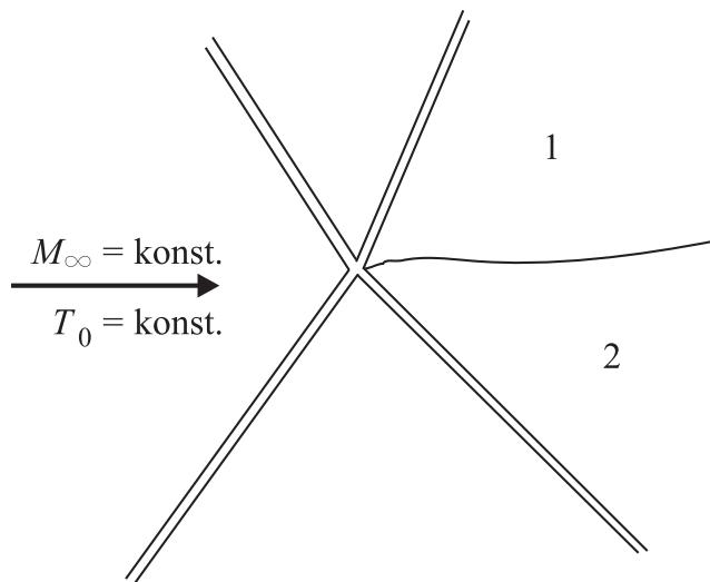
$$\gamma = 1.4 \quad R = 287 \text{ J kg}^{-1} \text{ K}^{-1} \quad p_{01}/p_{02} = 1.2 \quad M_1 = 1.6$$
