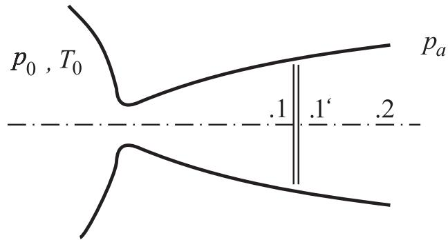
$$\begin{aligned} \dot{m} &= 200 \text{ kg/s} & T_0 &= 300 \text{ K} & p_0 &= 2.2 \cdot 10^5 \text{ N/m}^2 & p_a &= 10^5 \text{ N/m}^2 \\ \frac{p_{01}}{p_{01'}} &= 1.39 \text{ (ratio of total pressure across the shock)} & R &= 287 \text{ Nm/(kg K)} & \gamma &= 1.4 \end{aligned}$$
