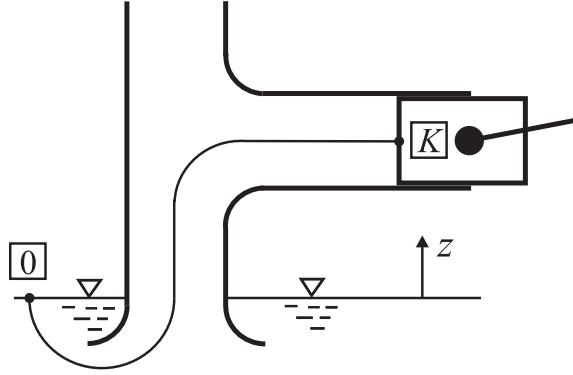
$$v_K = \frac{d\xi}{dt} = -\xi_0 \omega \sin(\omega t); \quad v_K^2 = \xi_0^2 \omega^2 \sin^2(\omega t)$$
