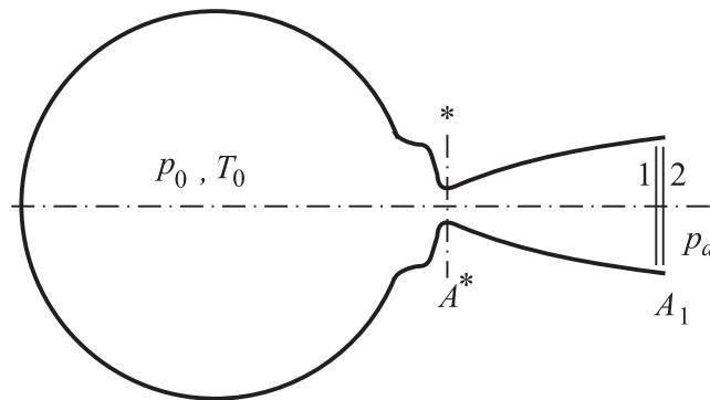
$$A_1 = 0.018 \text{ m}^2 \quad T_0 = 287 \text{ K} \quad A^* = 0.01 \text{ m}^2 \quad p_a = 10^5 \frac{\text{N}}{\text{m}^2} \quad R = 287 \frac{\text{J}}{\text{kg K}}$$
