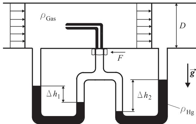
**7.2** Determine the pressure difference  $\Delta p = p_2 - p_1$  in the plotted bifurcation by neglecting the friction.
