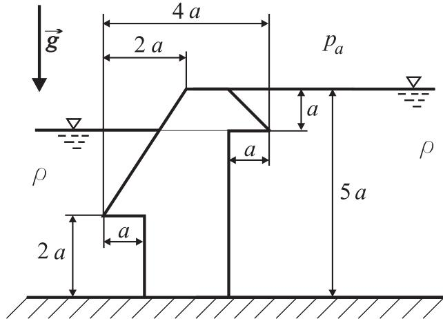
**5.6** A boiler with a small hole at the top is filled with water and is screwed on a plate.
