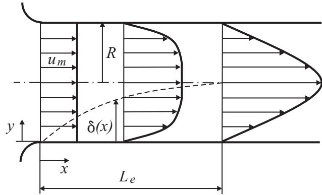
Determine in the inlet cross section, at the end of the inlet section and for  $\delta/R = 0,5$
