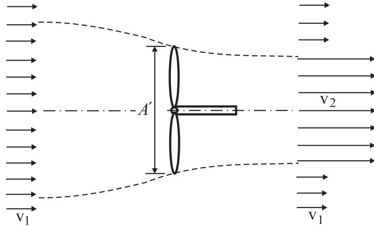
$$A' = 7,06 \text{ m}^2 \quad v_1 = 5 \text{ m/s} \quad v_2 = 8 \text{ m/s} \quad \rho = 10^3 \text{ kg/m}^3$$
