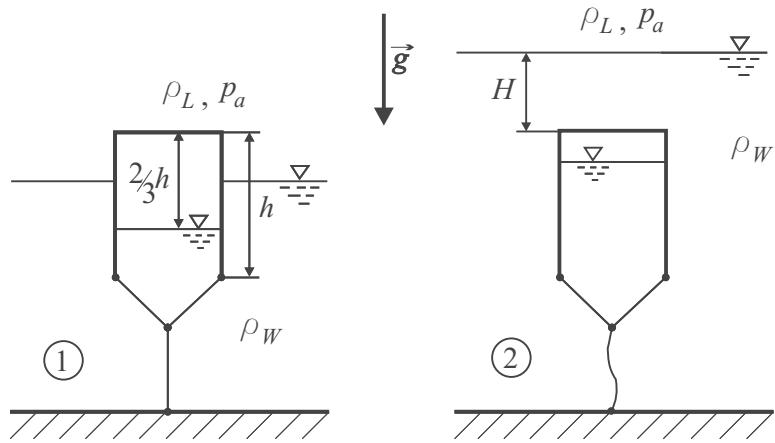
Hint: Assume, that the temperature inside of the buoy is constant and the enclosed air can be treated as a perfect gas. Neglect the weight of the cable.
