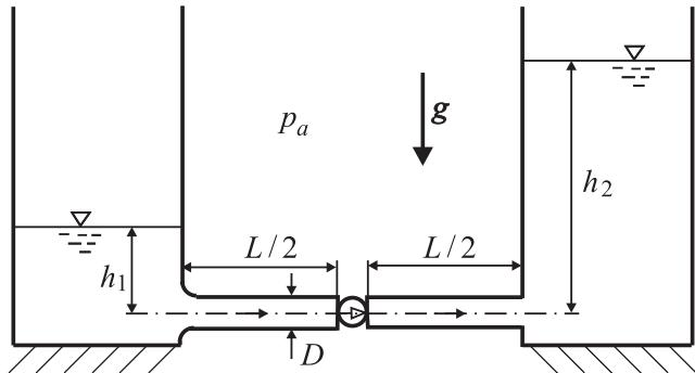
$$\begin{aligned} \dot{V} &= 0,63 \text{ m}^3/\text{s} & h_1 &= 10 \text{ m} & h_2 &= 20 \text{ m} & L &= 20 \text{ km} & D &= 1 \text{ m} & k_s &= 2 \text{ mm} \\ \rho &= 10^3 \text{ kg/m}^3 & \nu &= 10^{-6} \text{ m}^2/\text{s} & p_a &= 10^5 \text{ N/m}^2 & g &= 10 \text{ m/s}^2 \end{aligned}$$
