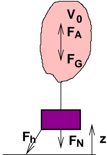
$$\begin{aligned}\sum F_z &= 0 = F_A - F_G - F_N - F_H \\ F_H &= F_A - (F_N + F_G) = \\ &= \rho_L(z=0)V_0g - mg = \\ &= (\rho_0V_0 - m)g = 10.6 \text{ N}\end{aligned}$$
