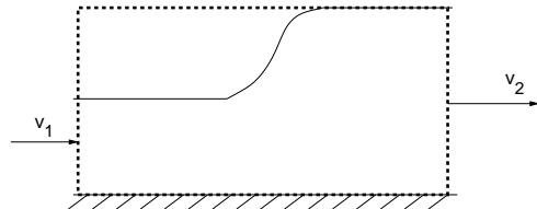
$$-\varrho v_1^2 z_1 b + \varrho v_2^2 z_2 b = b p_a (z_2 - z_1) + b \left( \int_0^{z_1} p_a + \varrho g z dz - \int_0^{z_2} p_a + \varrho g z dz \right)$$
