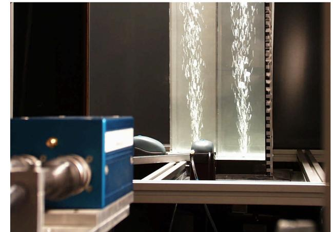
*Stereoscopic imaging of bubbles rising in water to study bubble cloud dynamics and turbulence production in multiphase flows*
