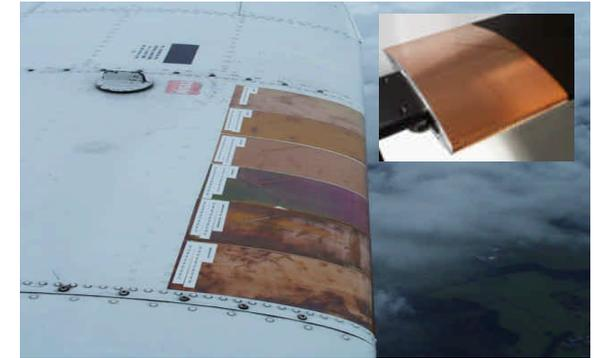
*Free flight measurements using multisensor hot-film arrays at 130 knots and an altitude of 3000 m.*
