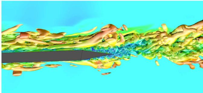
*LES of the turbulent flow around a sharp trailing edge to predict noise radiation.*
