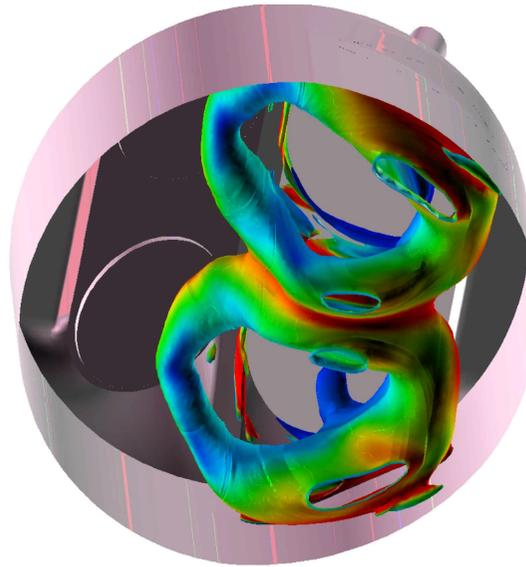
*Ring-like vortices within the cylinder of a 4-valve piston engine*
