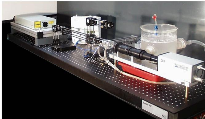
*Optical set-up to apply for DPIV measurements in a micro-axial blood pump rotating at 33000 rpm*
